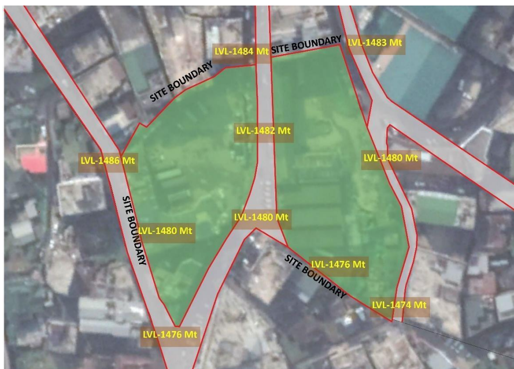
Figure 9 The spot levels of the proposed site for the Business cum Tourism and Cultural Centre
