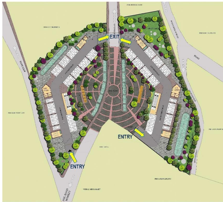
Figure 26 Circulation Zones on the G.F. of the proposed layout of the Business cum Tourism and Cultural Centre
